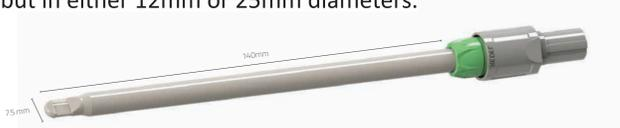
The new Futura PICO system launched at BPI Boston in 2017 has a unique, patented 7.5 mm diameter probe that can be autoclaved or steam sterilized in situ. The four pure platinum electrodes are beneficially positioned to maximize the current path between the electrodes around the tip of the probe body and produces a smaller symmetric field of measurement compared to other capacitance based probes, while having a comparable performance to other probe configurations in the Aber range (Fig. 1a & b).
